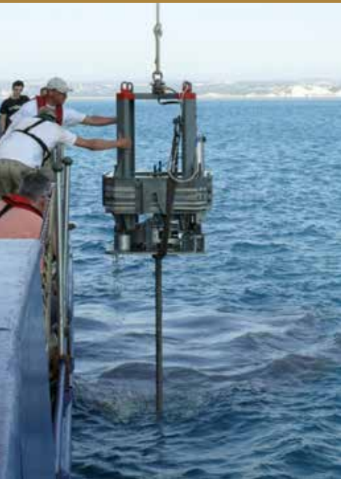
Deployment of the MARUM long-term piezometer from research vessel POSEIDON to monitor indicators for sub-seafloor deformation and fluid flow in the slope offshore Nice, France. This slope collapsed in 1979 and caused a major landslide and tsunami. The governing geoprocesses that caused this catastrophic event are studied by MARUM researchers.
