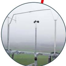
Solution with high-voltage-resistant insulated HVI®power Conductor for conducting lightning currents safely past sensitive components.
