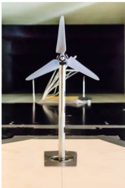
Wind turbine model using a gimbal support to simulate simplified floating platform
