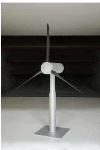
Model wind turbine with active load and pitch control
