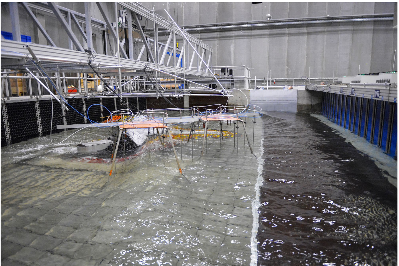
Testing of breakwater for Port of Hanstholm (19.01.2018).
