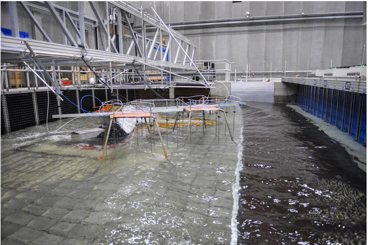
Testing of breakwater for Port of Hanstholm (19.01.2018).
